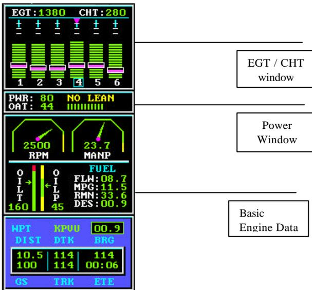
The Fuel panel in the lower-right corner of the Basic Engine Data Window has four values:
