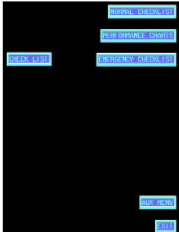
Items on the Normal Checklist submenu display a toggle page with check-off items. Colors are used to distinguish lines of text. Item headings appear in cyan. Current item selection appears in magenta. Items that are checked-off display in green with a check mark next to the line. Press **PREV** or **NEXT** to move to the desired item. When completed, press **DONE** to toggle the line to green. Pressing **DONE** again toggles the line back to normal or unchecked.
