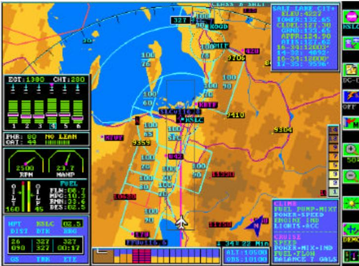
The mapping window is the main screen and largest window. It contains the graphical display of the aircraft's position in relation to items such as airports, navaids, special use airspace, and geographical information. It also contains the graphical ICONs that provide hot key access to the functions available to the pilot.
