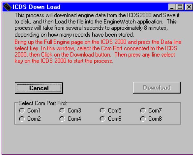
Start the EngineWatch application from a PC, until the ICDS Down Load Screen appears (shown above). Follow instructions found in the Help functions of the EngineWatch software to transfer the data from the ICDS 2000.
