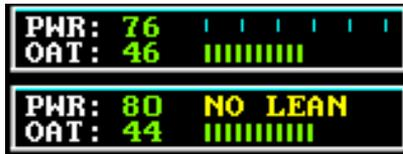
**OAT** – Outside air temperature in degrees Fahrenheit, derived from electronic probe installed as part of the engine-monitoring module. This OAT value does not replace the factory installed and certified Outside Air Temperature gauge, and is only used for the %PWR calculation.
