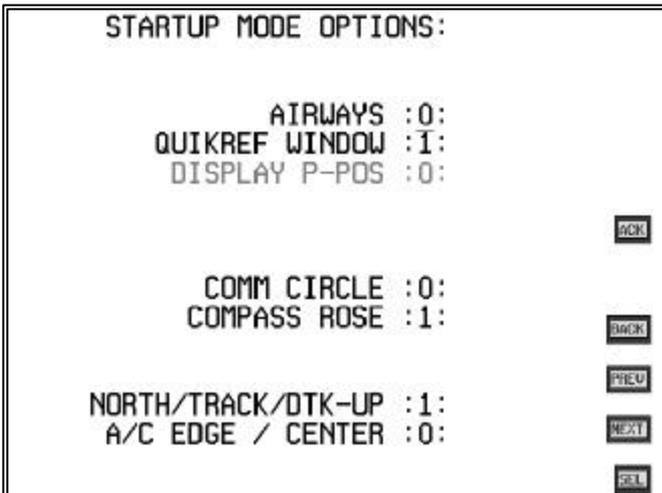
**Airways** – Enter 1 to have airways display on startup or enter 0 to not display airways on startup.
