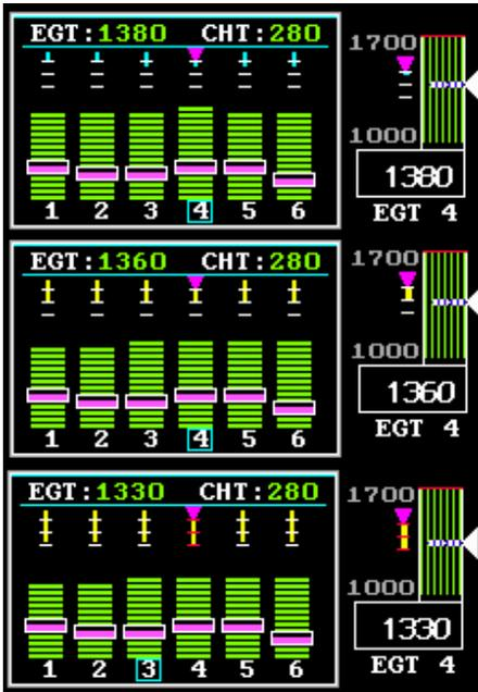
The sequence shown here from top to bottom is 25, 50, and 75 degrees down from peak EGT.
