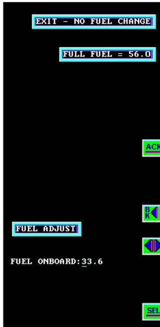
The pilot may **ACK**nnowledge (LSK-5) the fuel amount shown, or use the <> keys to increment or decrement the fuel onboard. LSK 2 will allow the pilot to accept the default full fuel amount for the aircraft with a single key press.
