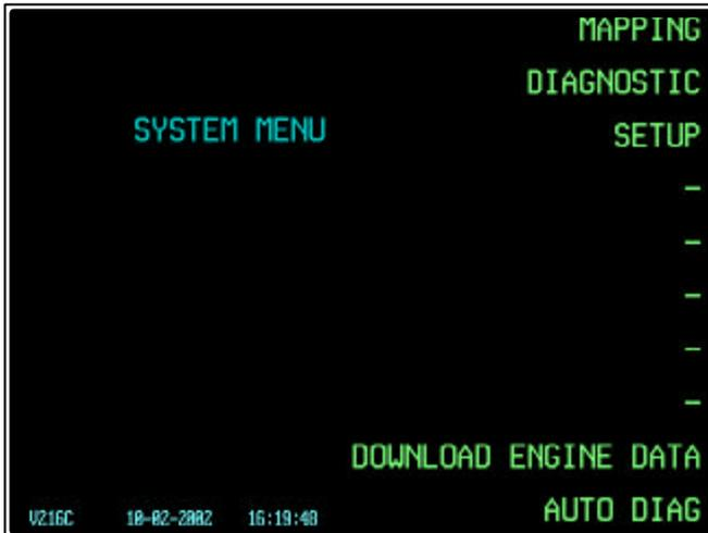
This guide is intended to familiarize the pilot with the setup options available with the ARNAV ICDS 2000 Revision BH software. Power up the ICDS 2000, and at the SYSTEM MENU prompt, press LSK-3, SETUP.
